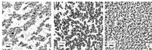
**Figure 1** Images containing CNT: (a) Frozen sample (b) at room temperature (c) at 100°C [15]
